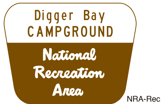
Figure 7-7 —Example of signing for recreation sites within a congressionally designated special area.
