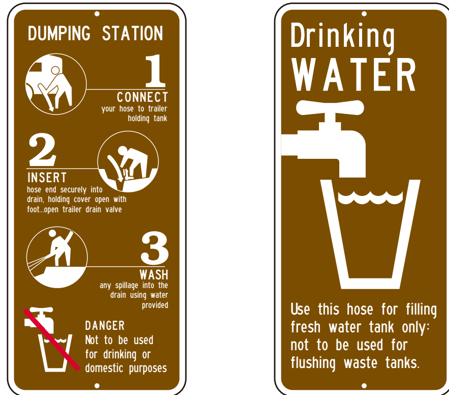
Figure 7-4 —Sanitary dumping site signs.
