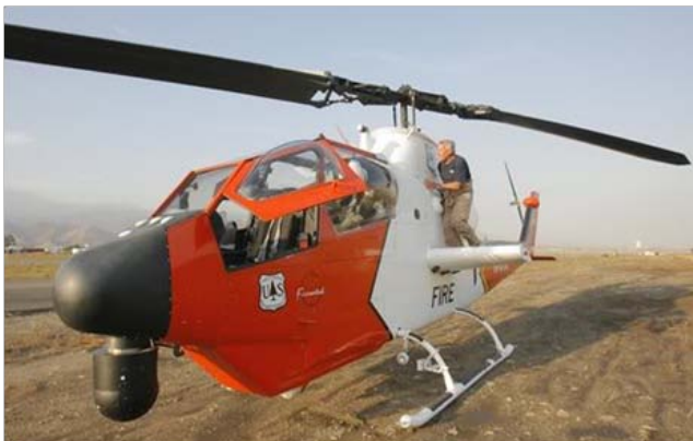
Pilot readies a U.S. Forest Service Cobra helicopter outfitted with video and infrared cameras. The two-seat helicopter flies above fires and beams real-time images of forest terrain and 'hot spots' to fire commanders. (AP Photo Jae C. Hong)
