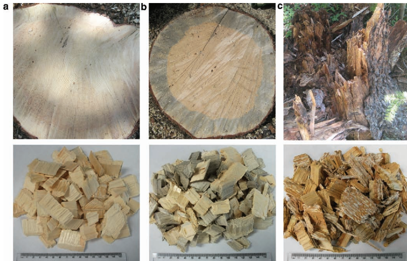
Figure 1. Pictures of tree stem and wood chips from selected live and beetle-killed lodgepole pine trees used in this study. (a) BL; (b) BD4; (c) FDD.
