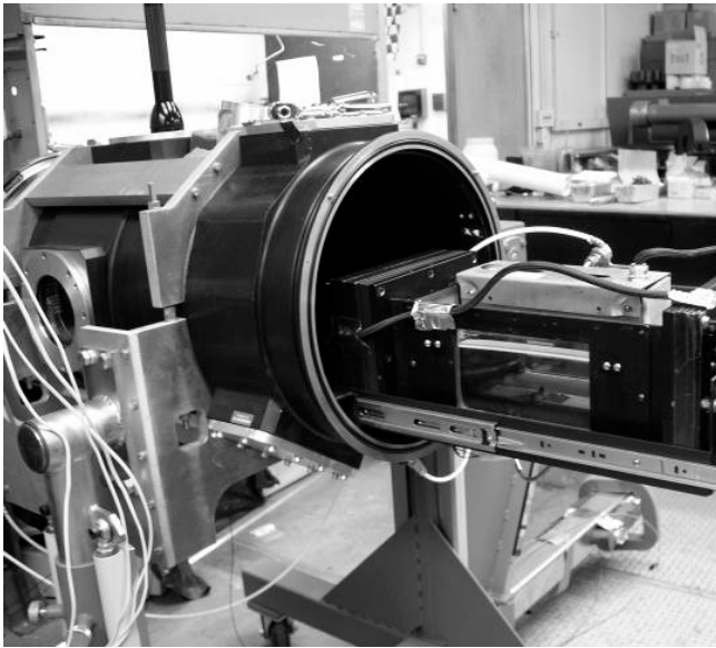
Figure 2. Photograph of the FIST tunnel in the containment chamber.
