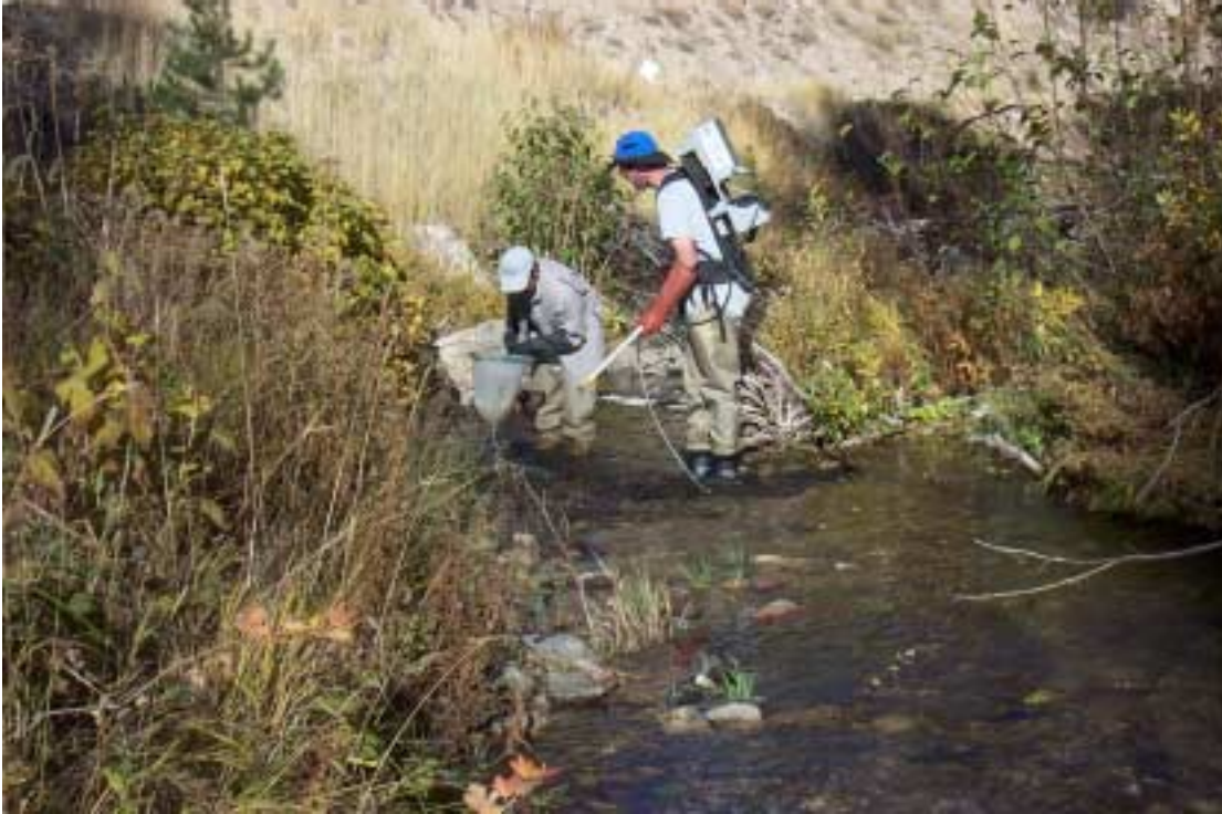
Figure 3. Sampling fish in the North Fork Boise River basin using backpack electrofishing.
