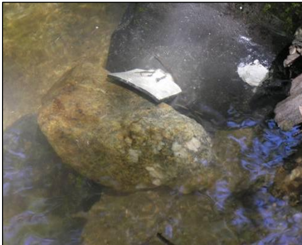
Photo 12. Temperature sensors glued to rocks in mountain streams - notice the rocks propped against the front of the sensors to hold them in place while the epoxy sets. (a) A sensor with a neoprene flap, and (b) a sensor in a canister. Smaller prop rocks than that shown in (a) are typically used because only a small amount of pressure is needed.
