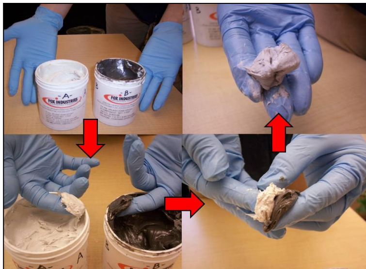
Photo 6. Preparing the Fox epoxy for use involves extracting equal amounts of each component and mixing together for one minute until the color is uniform throughout. Fingers should be wetted before and during handling the epoxy to minimize messiness.
