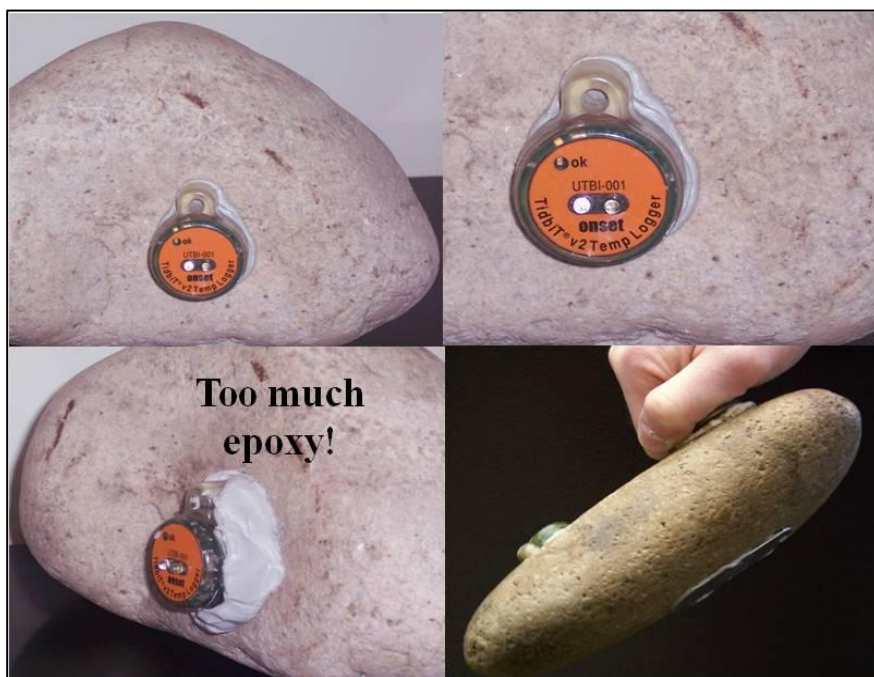
Photo 8. Temperature sensor attached to rock surface with the Fox epoxy in a laboratory setting. Once the epoxy fully sets, the sensors are cemented to the rock surface. Lower left panel demonstrates applying too much epoxy to attach the sensor, which would prohibit data retrieval with an underwater shuttle. Lower right panel shows a 5 pound rock held aloft by the sensor.
