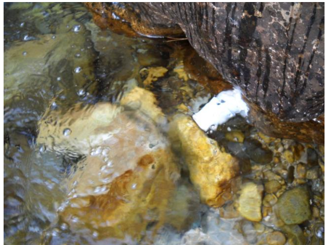
Photo 12. Temperature sensors glued to rocks in mountain streams - notice the rocks propped against the front of the sensors to hold them in place while the epoxy sets. (a) A sensor with a neoprene flap, and (b) a sensor in a canister. Smaller prop rocks than that shown in (a) are typically used because only a small amount of pressure is needed.
