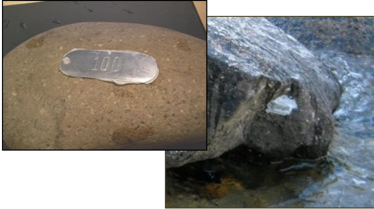
Photo 13. Metal forestry tag attached to a rock using Fox epoxy to monument the location of a stream temperature sensor.
