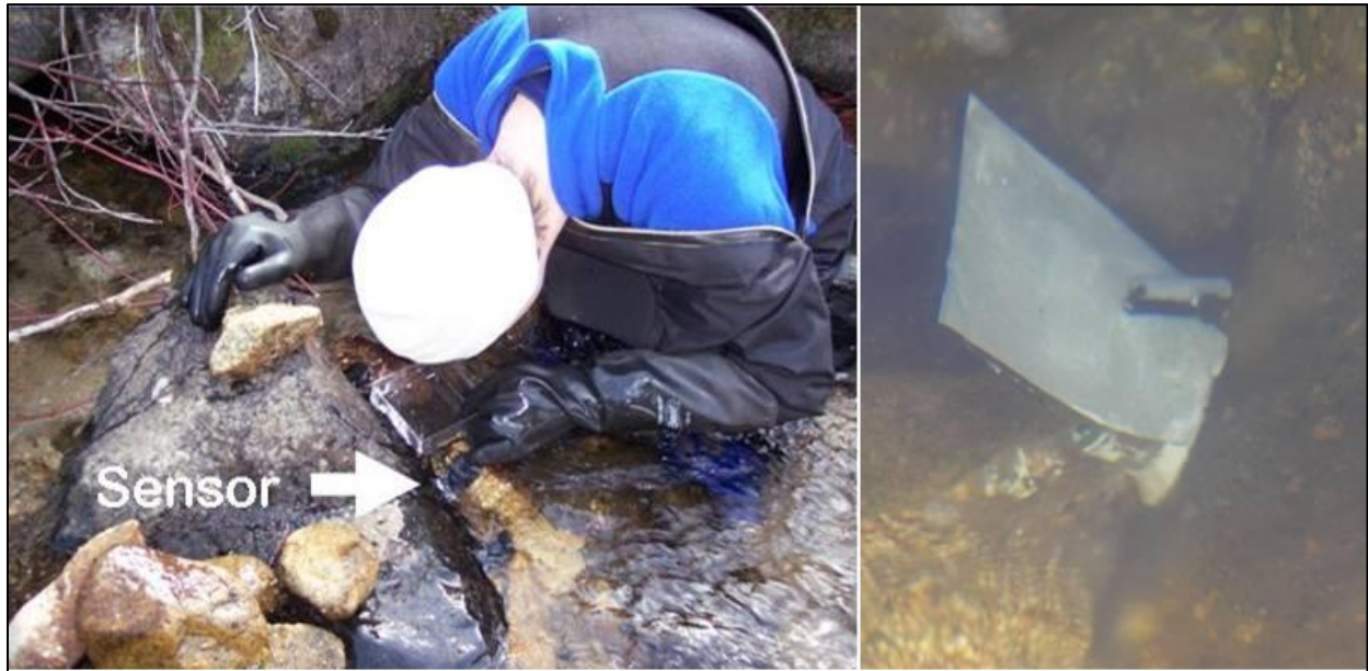
Photo 11. Inspecting a temperature sensor attached to a rock surface using a viewing box in the field. No gap should be apparent at the contact point between the epoxy and the rock surface.
