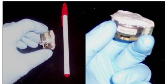
Photo 7. Fox epoxy applied to the back of a temperature sensor ready for deployment. Enough epoxy should be applied that it can cover the surface of the sensor to a depth of approximately 1/8 inch.
