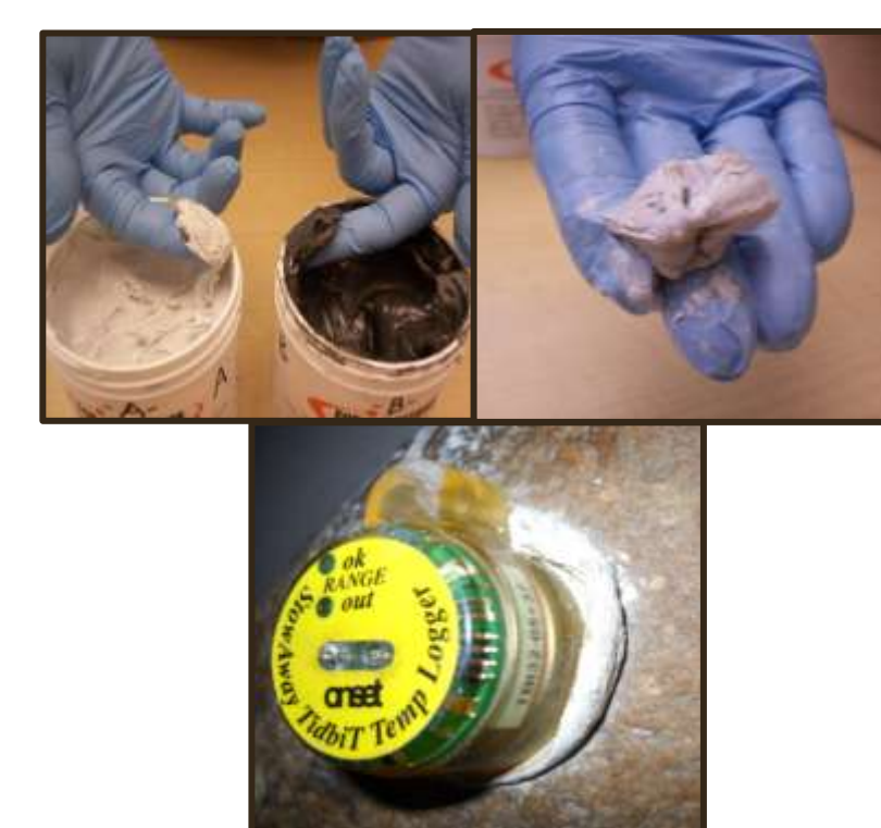
Figure 3. We mix a 2-part epoxy to use on sensors that are then attached to large rocks in streams.
