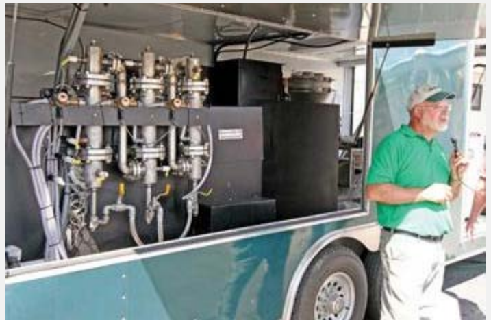
Phillip Badger, president of Renewable Oil International Inc., talks about the first pyrolysis process Monday during a presentation near Heppner, Ore. The trailer behind him is a self-contained unit which can convert woody materials into bio-oil, bio-char and synthetic gas. U-B photo by Andy Porter
