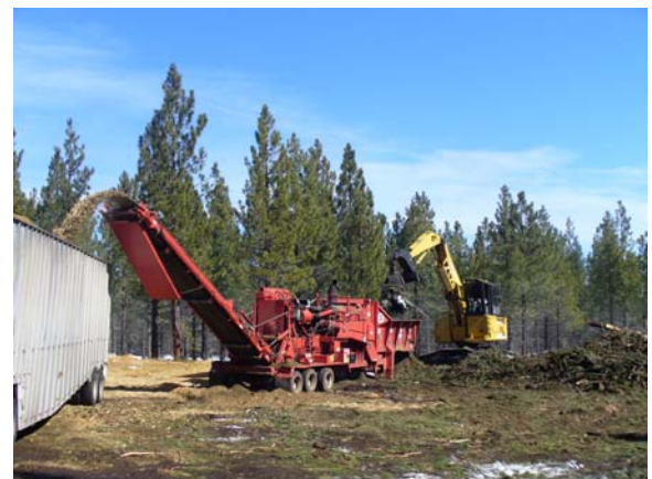
Figure 3. Grinder creating wood chips for local co-generation plant.
