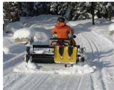
Juneau Nordic Ski Club volunteer ski trail groomer smoothes skate skiers' trail in Mendenhall Campground on February 22. The device used to cut the classic cross-country track is suspended above the snowmobile's raking implement.
