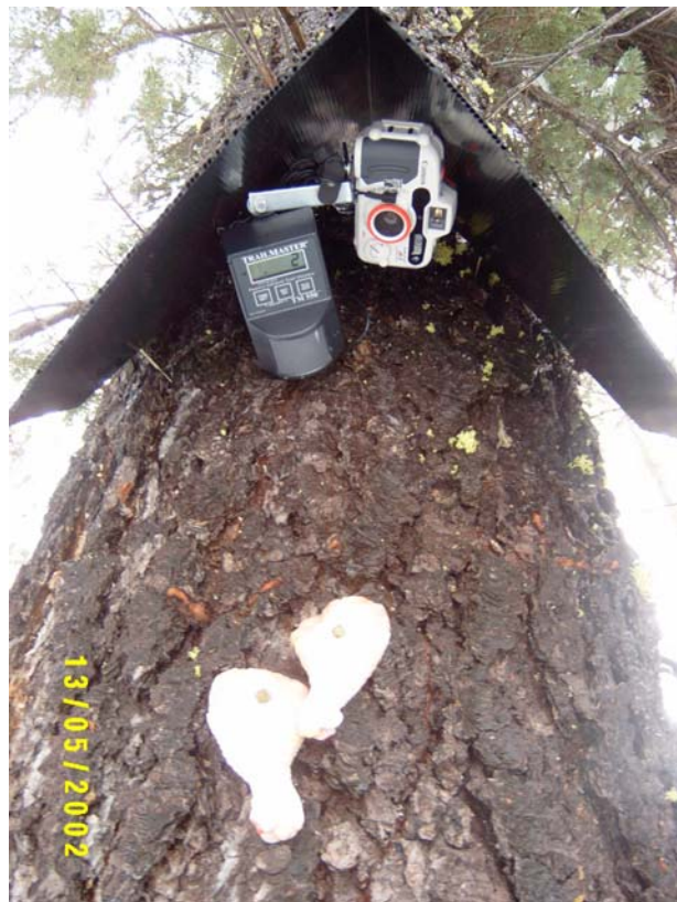
Figure 4. Photograph of Trailmaster 1500 (above) and 500/550 (below) camera configurations.
