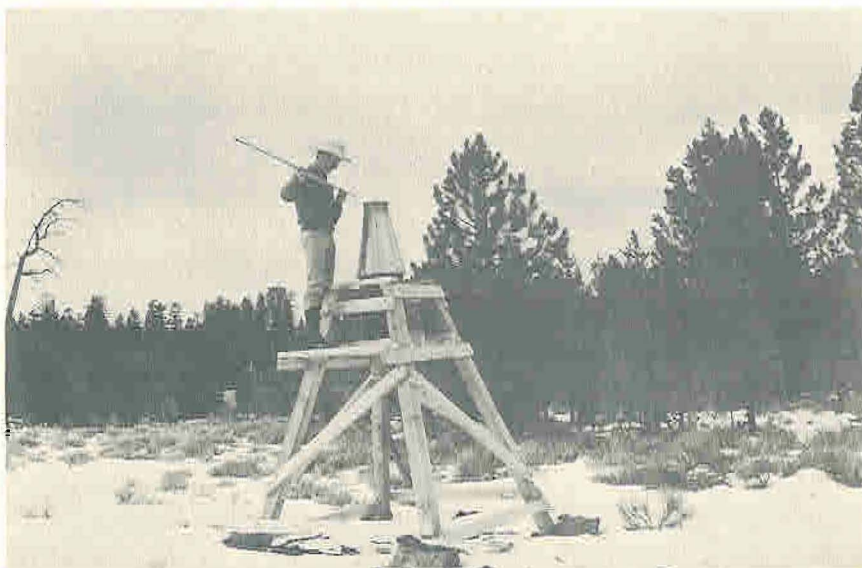
Figure 2.--Stick measurements of the gage contents give periodic records of accumulated precipitation.
