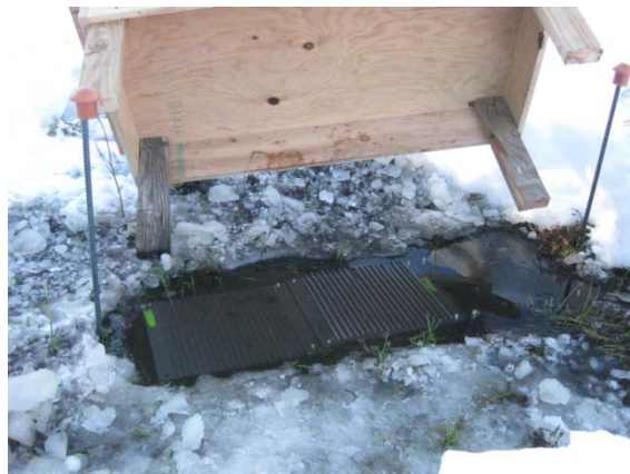
Photo 4: Field installation of biofilm plates, shown with wood cover to keep snow off biofilm.
