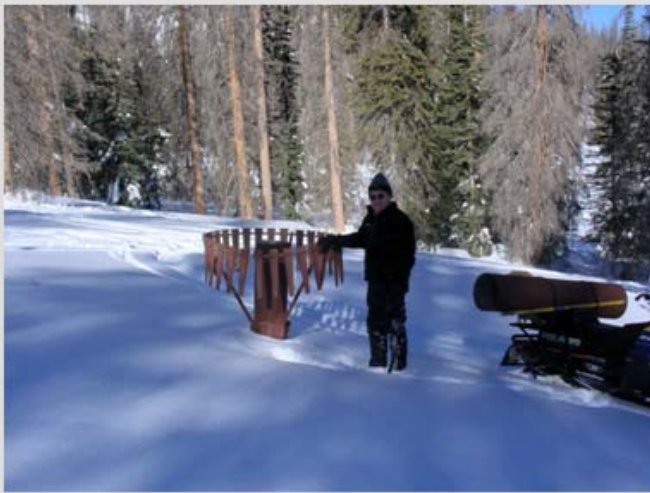
A 3.7 meter gage about to be extended in Southwestern Utah 1/19/05. (NRCS)
