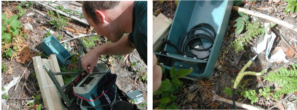
Figure 6. Sampling soil moisture using time domain reflectometry (TDR).
