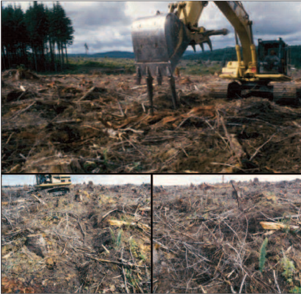
Figure 14—Tillage with an excavator in plots with soil compaction (top), and traffic lanes before (bottom left) and after tillage (bottom right) at the Fall River research area.
