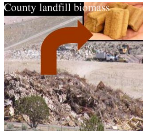
Carson City, Nevada, landfill waste wood pile, and pellets manufactured from chipped wood.
