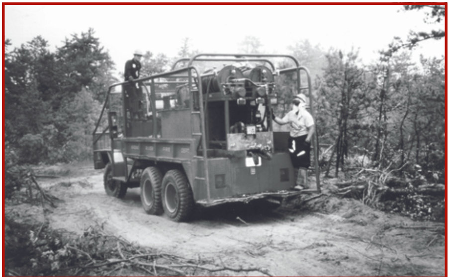
Figure 12—Firefighters who ride outside an engine can be killed when they are thrown off or when the vehicle rolls.
