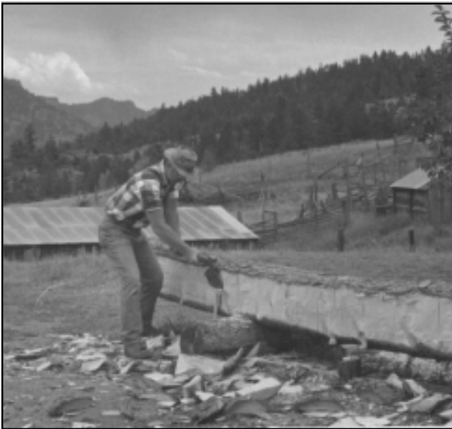
Figure 2—Barking your knuckles comes with the territory when you choose to hew logs with a broad ax.
