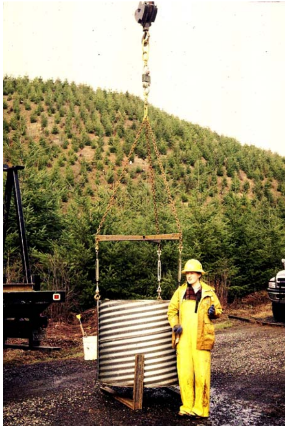
Figure. 9. Detail of tank lifting, leveling and weighing apparatus used with the crane.
