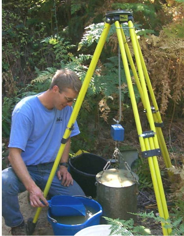
Figure 7 The tripod sediment determination system shown using a 100lb (45 kg) capacity load cell and a fiberglass survey tripod.
