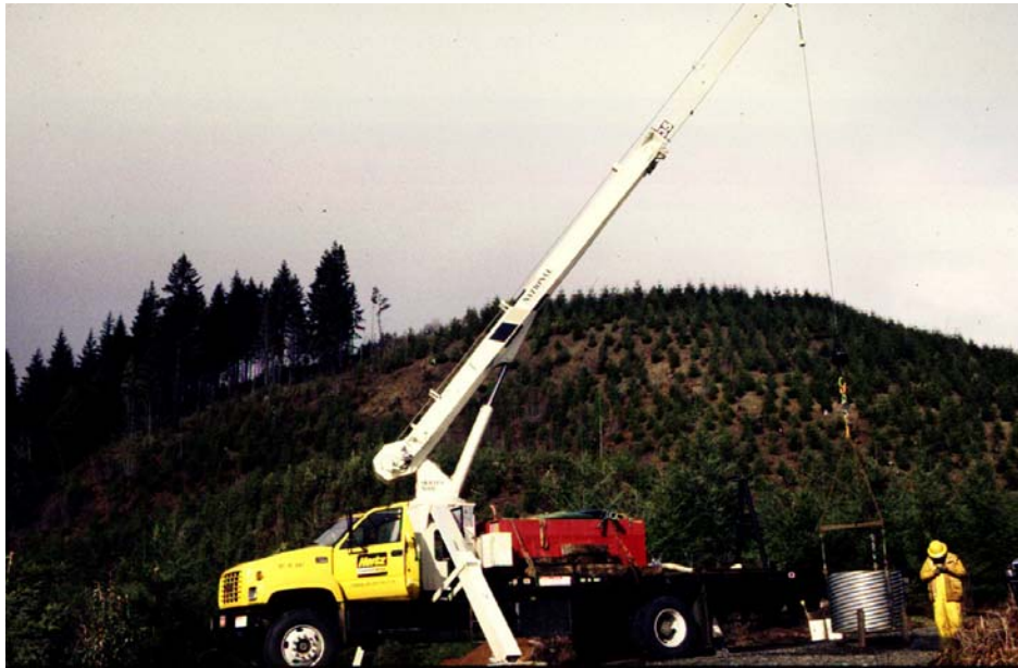
Figure 8. Crane and load cell system used to weigh large sediment samples. Water supply tank is mounted on the bed of the crane
